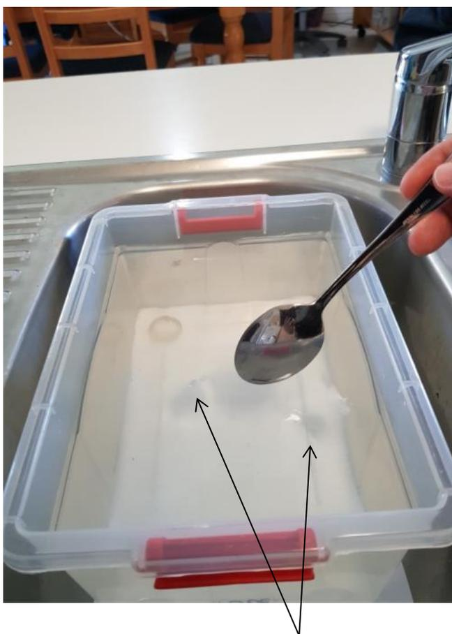
Picture 1 - note two vortex shadows in the tub? There's a half torus vortex there for sure!
