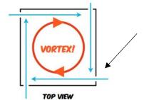
**Note:** Ensure the vertical air slits are located diagonally opposite each other, to allow the air to circulate. Air will able to flow in through the slits in the direction of the blue arrows, when the fan is turned on.
